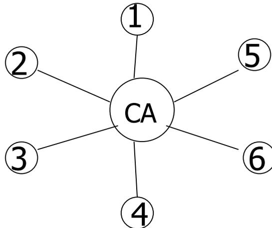
If a new node is inserted in the network, only that new node and the CA need to be configured with the public key for that node
